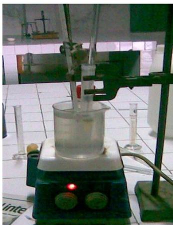
Fig 1: Micro melting Test Apparatus
